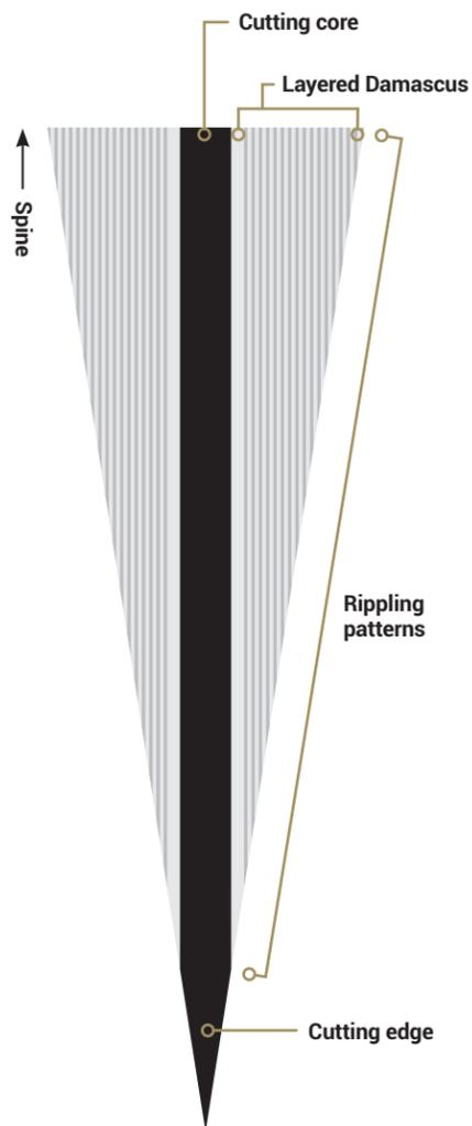
Shun's Damascus is formed by layering different types of metal alloys together, then forging them into a single piece. The process and the different characteristics of the layered metals create the rippling patterns you see on the blade. The number of layers can vary; many Shun knives, for example, have 34 layers of metal on each side of a high performance VG-MAX cutting core.
