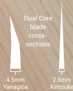
The Shun Dual Core Yanagiba has the length, weight, and single-bevel design of a traditional Japanese yanagiba. The blade stock is thicker than the rest of the Dual Core series (4.5mm vs 2.5mm). This gives the knife heft and rigidity to glide through cuts with ease. This single-bevel blade offers a strong, razor-sharp edge and simplified sharpening. A gentle hollow-grind on the back of the blade makes food release easier.
